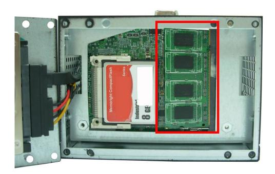
(B) Press down the memory module then check dimm holder hook well.
