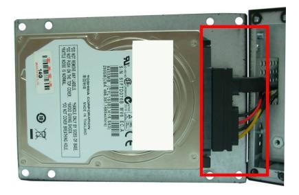
5. Turn the chassis shield screws with the hanging holders to tighten well.
