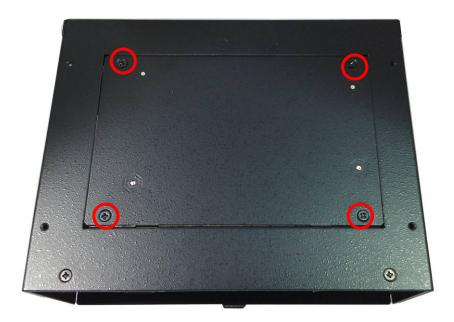
11. Put the top Chassis shield back and screw on as indication of the picture below.
