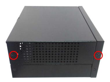
2. Push the Chassis shield towards the back then open it.
