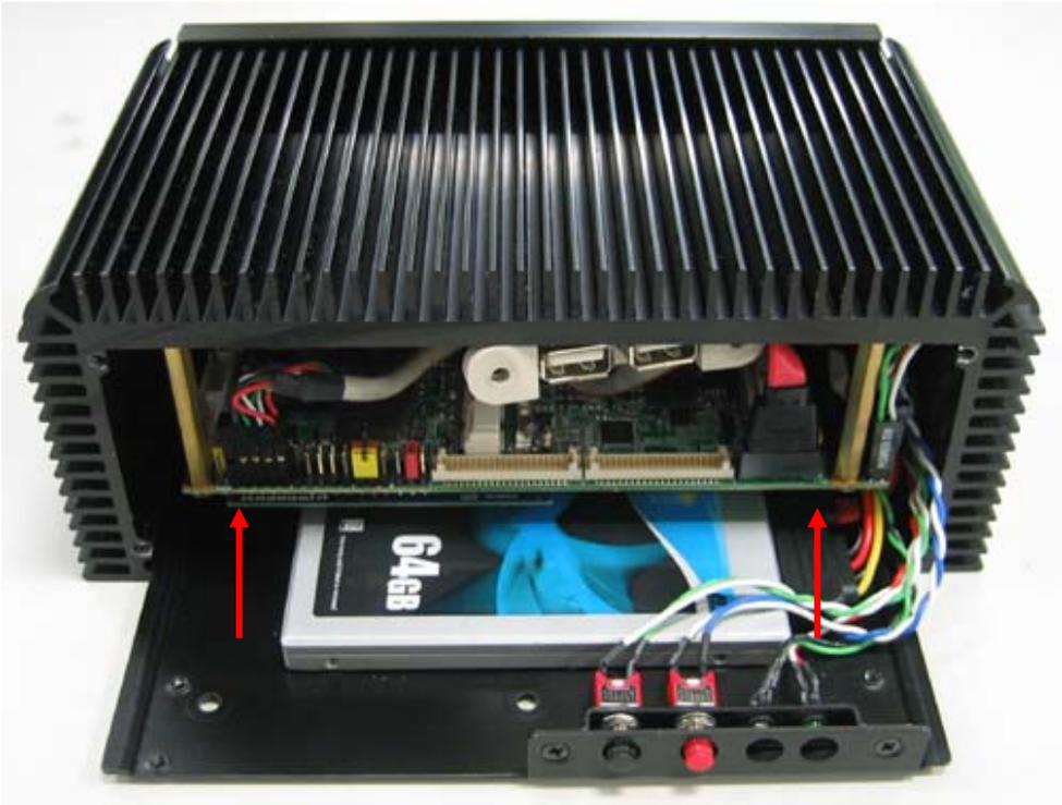
11. Lock the USB cable screws , put back the front panel , final lock the front panel screws.
