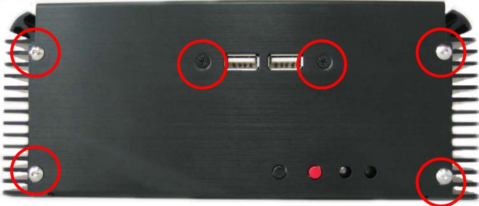
11. Lock the chassis foot screws.
