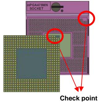
4. Socket P has 478 pins, but is not pin-compatible with Socket M CPU.
