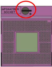
1. Use the flat-type screw drive to unlock the CPU socket
