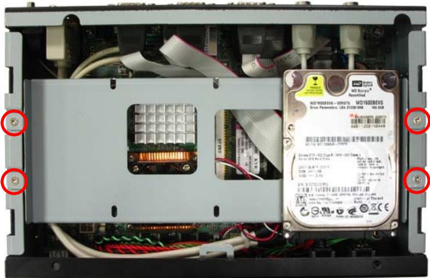
8. Push the Chassis shield towards the back then open it.
