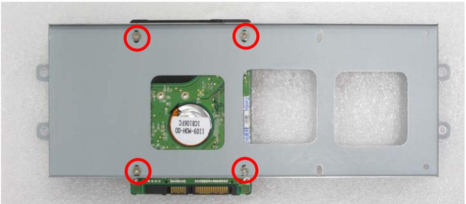
7. Screw on as indication of the picture below Turn the screws.
