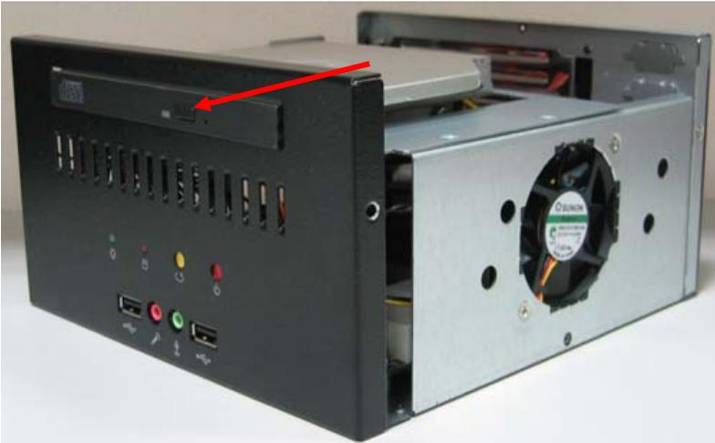
17. Turn the chassis shield screws to tighten well.
