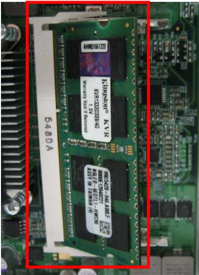
6. Press down the memory module then check dimm holder hook well.
