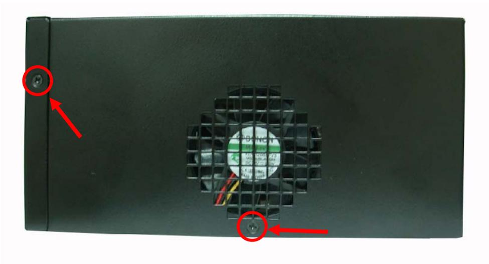
2. Push the Chassis shield towards the back then open it.
