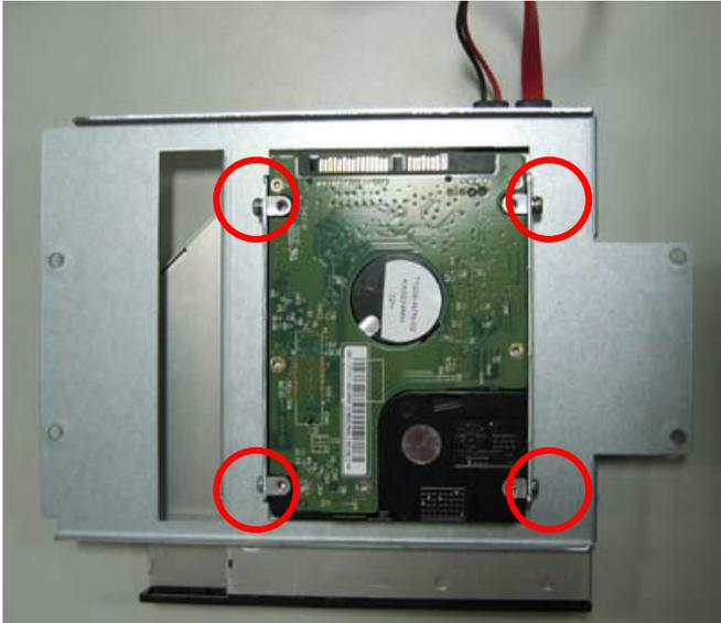
15. Connect SATA cable from motherboard to the HD drive, then connect the ATX output (15-pin).
