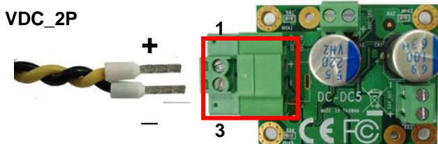
VDC\_2P: Terminal Block 2-pin power connector
