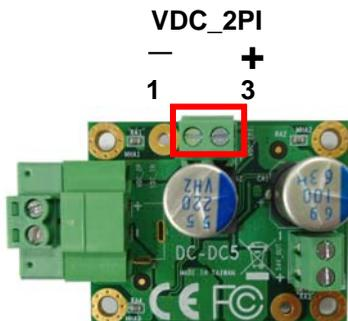
VDC\_2PI: Terminal Block 2-pin power connector
