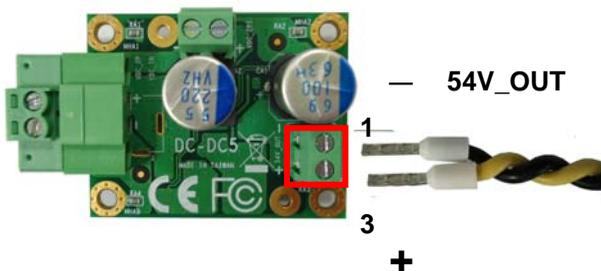
54V\_OUT: Terminal Block 2-pin power connector
