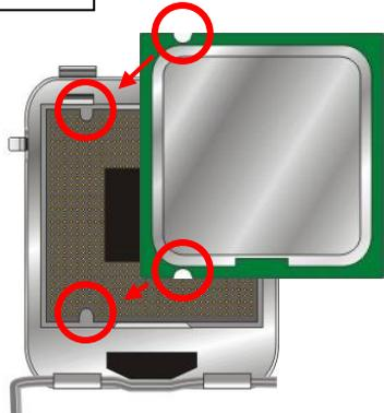
3. Place the CPU on the top of the pins
