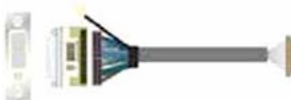
DVI Module With DVI Cable x 1 (BADPDVIP_A&OALDVI-DF13) (4120008011&1040483)
