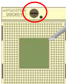
Socket479 for Intel Pentium M/Celeron M With 478-pin PGA
