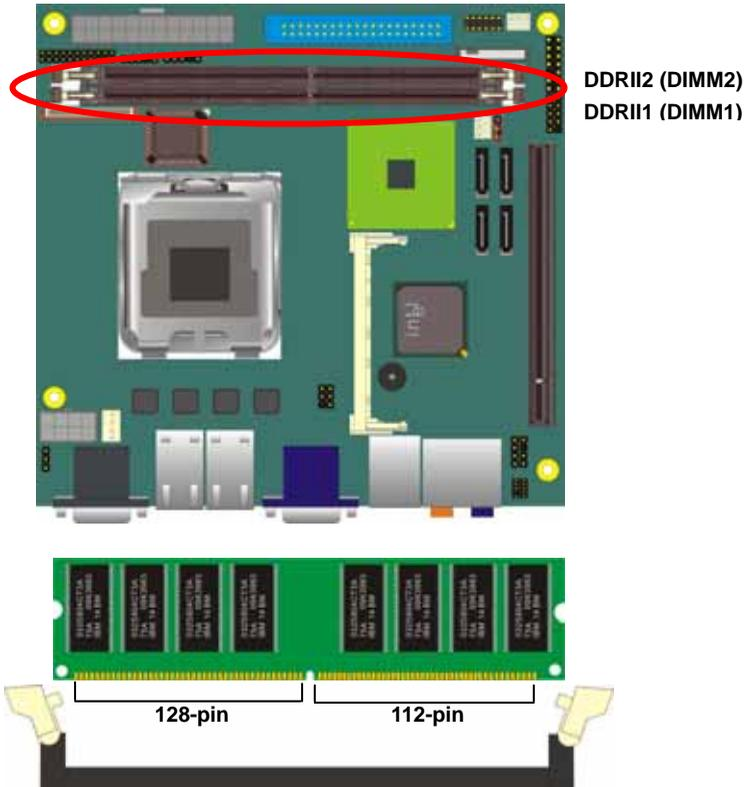
Please check the pin number to match the socket side well before installing memory module.
