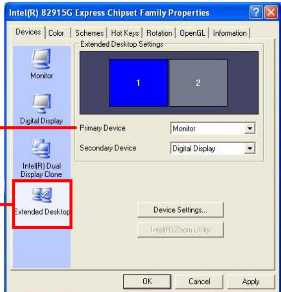
**Notice: The dual display needs PCIE-SDVO module to support more than one display devices.**
