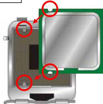
3. Place the CPU on the top of the pins
