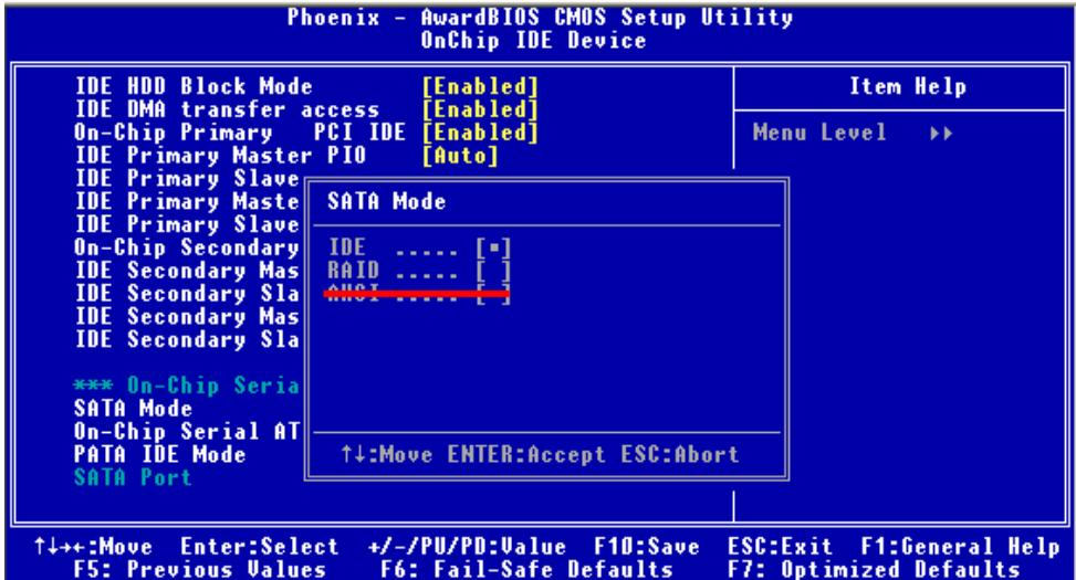
This option can let you select whether the Serial ATA hard drives would work under normal IDE mode or RAID mode. The RAID mode need more than one HDD is applied.
