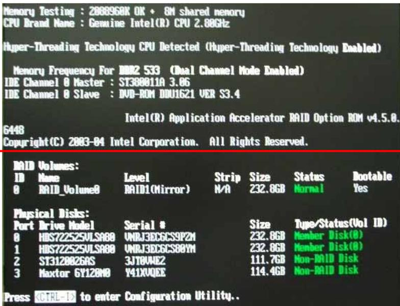
Once you enable the RAID mode, the boot-up screen would pop up the RAID configuration option for setup.
