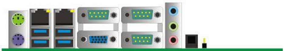
PS2 USB_RJ45_1/2 COM1 + CRT COM3+COM2 Audio SPDIF
