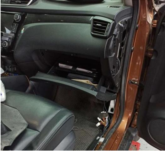
1. Find the air intake (white) behind the glove compartment.
