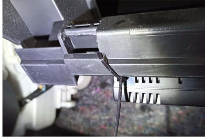
4. Fix it with cable ties behind glove compartment
