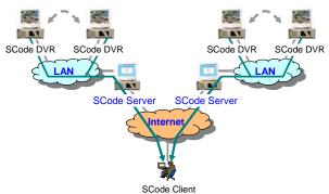
One SCode DVR can be monitored and controlled by multiple remote SCode Clients from different networks, simultaneously.
