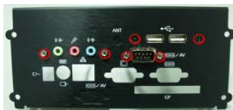
3-5 Connect Audio , USB , DB9 cable with MB
