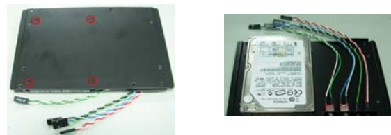
3-6 Screw MB into Copper Pillar
