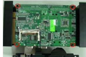
3-6 Screw MB into Copper Pillar
