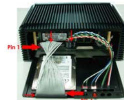
3-8 Connect HDD cable and Power / Reset button
