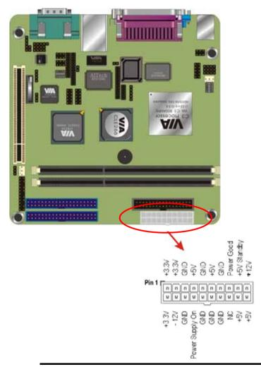
Warning: Incorrect installation of the power supply could result in Warning: serious damage to the motherboard and connected peripherals. Make sure the power supply is unplugged from the AC outlet before connecting the leads from the power supply.
