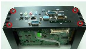
3-8 Connect HDD cable and Power / Reset button
