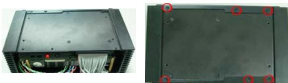
3-10 Assemble Front plate and lock
