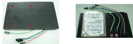
3-5 Connect Audio , USB , DB9 cable with MB
